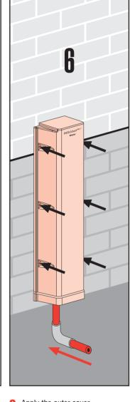
Locate water service pipes and select location for INSUduct as required. Open the packaging and put press firmly on to the aside screws and fixings for future use. Remove back plate (black plastic) and offer to wall or post. Mark fixing points (a minimum of 4 is required). Put aside the back plate and drill the wall with a 6mm drill bit. Insert wall plugs and then fix back plate to wall / post with the screws provided (38mm No.10).
