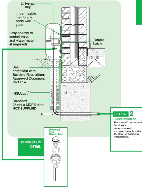
Failure to install Groundbreaker to this specification will eliminate the manufacturers guarantee and may result in a water company refusing to connect the water service
